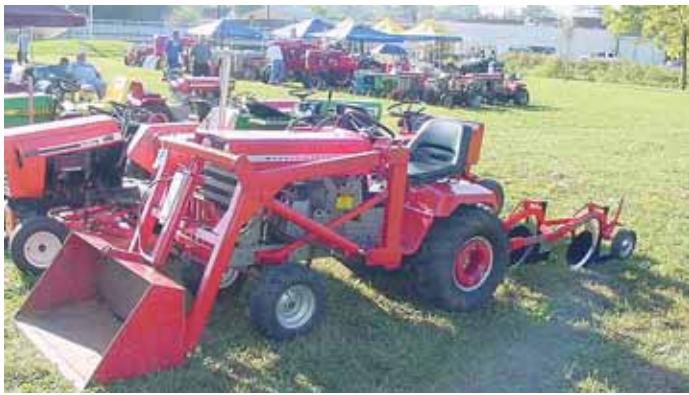
"I use it to clean out our 48-in. wide baby calf stalls," says Daniel Perkins, who built this front-end loader from scratch for his Massey Ferguson 1650 garden tractor.
