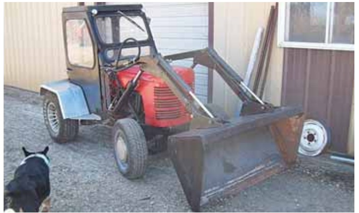
Richard Kast built his loader tractor around a 4.3-liter engine from a 1987 GM pickup and a 4-speed transmission from a 1957 Chevy pickup.
