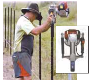
Hammer action on this handheld post driver is provided by a Honda GX35 gas engine, eliminating the hoses needed for hydraulic or air-powered drivers.
