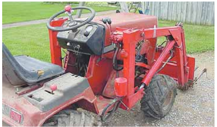
Loader's 2 1/4-in. dia. lift cylinders came off a New Idea hay baler.
