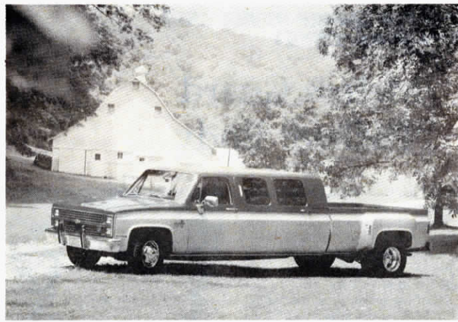
Standard 1-ton Silverado pickup is lengthened almost 4 ft.
