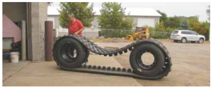
Truck tires drive 25-in. wide rubber tracks. Computer control of the four drive wheels provides precise control of slippage, constantly adjusting power from side to side.
