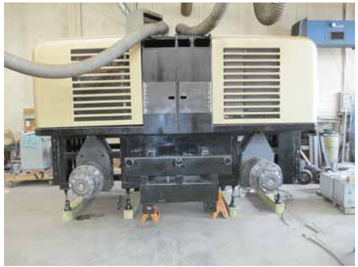
Tractor is driven by electric wheel motors, powered by 202 hp diesel generators. Its main drive system was fashioned after General Electric railroad engines.
