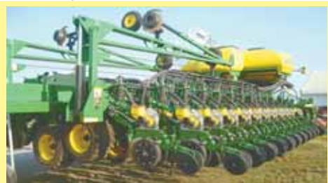
Stine Seed Company used this custom-built 60-row planter to test high-density corn hybrids, which were planted in 12-in. rows and spaced 12 in. apart in the row.
