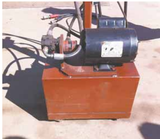
Gene Luoma's portable hydraulic power unit is powered by a 1 hp single phase electric motor and designed to run any tools that need a hydraulic power source.
