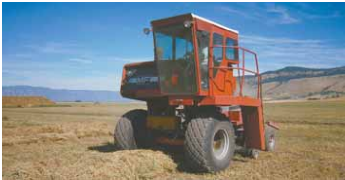
Howard Elmer and his son converted a 1980's model Massey 550 combine into this self-propelled baler, cutting the combine frame off behind the cab.
