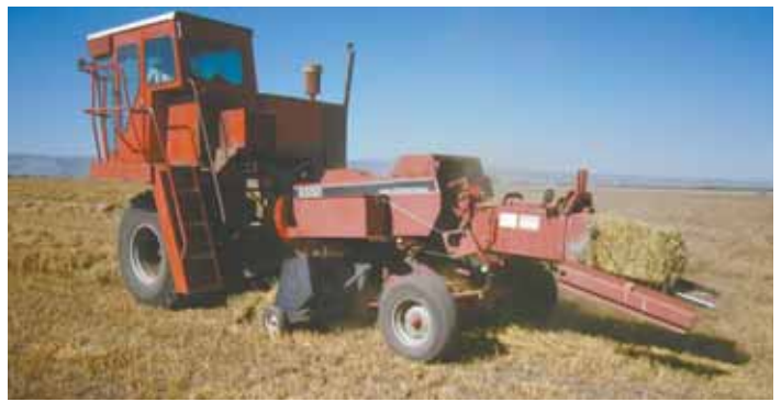
They cut 3 ft. off the tongue of an IH 4650 in-line baler and coupled the 2 implements together. The combine engine powers the baler through a right angle gearbox.
