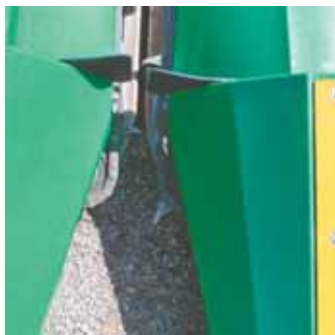
Corn Stalk Guide attaches to plastic header snouts, guiding stalks past the gathering chain and idler sprocket. Ears move smoothly into head without bouncing away.
