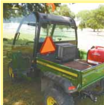
Gary Holloway mounted a small air conditioner and Honda generator in his Deere Gator, cutting an opening on back of the cab to install the AC unit.
