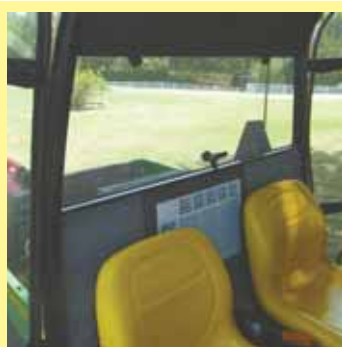
Gary Holloway mounted a small air conditioner and Honda generator in his Deere Gator, cutting an opening on back of the cab to install the AC unit.
