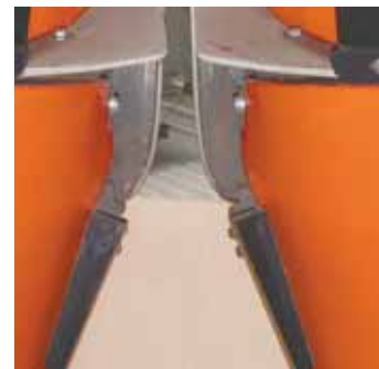
Corn Stalk Guide attaches to plastic header snouts, guiding stalks past the gathering chain and idler sprocket. Ears move smoothly into head without bouncing away.
