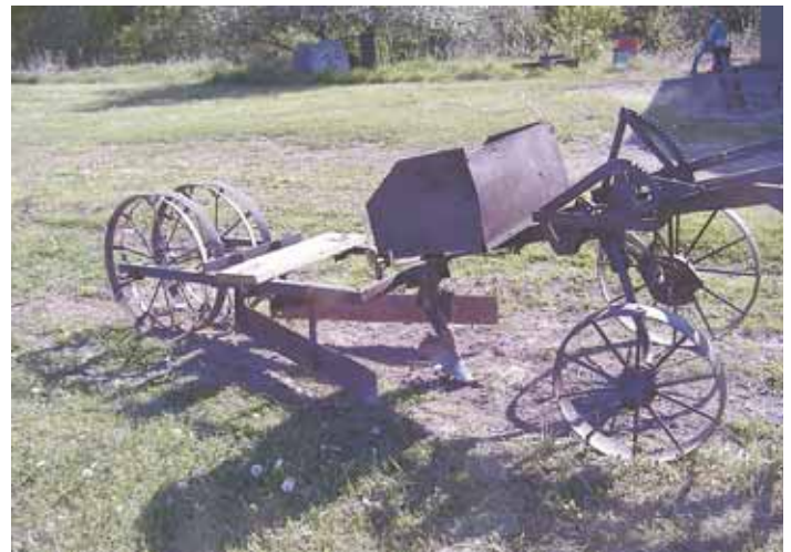
Bob Fredrickson converted a 1940's vintage, one-bottom plow into this slick berry planter. Wooden plank seat mounts just ahead of plow's packer wheels.
