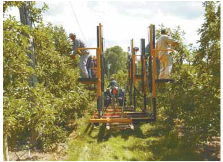
Work platform has 2 stations that run separately off tractor hydraulics. Stations go up and down and in and out, allowing workers to do a variety of jobs on fruit trees.
