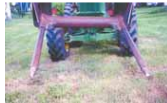
Bale fork uses 5-ft. long steel pipes supporting 8-in. long solid steel spindles ground down to a point (left). Bucket teeth were made out of truck leaf springs.
