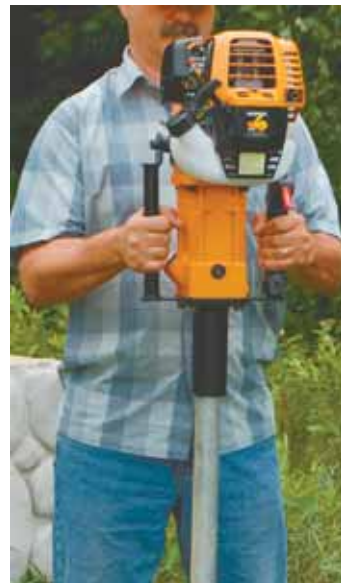
Ultra-Driver gas-powered post driver burns less than a quart of fuel per hour while delivering 1,100 blows per minute.
