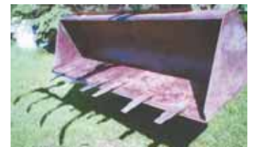
Bale fork uses 5-ft. long steel pipes supporting 8-in. long solid steel spindles ground down to a point (left). Bucket teeth were made out of truck leaf springs.
