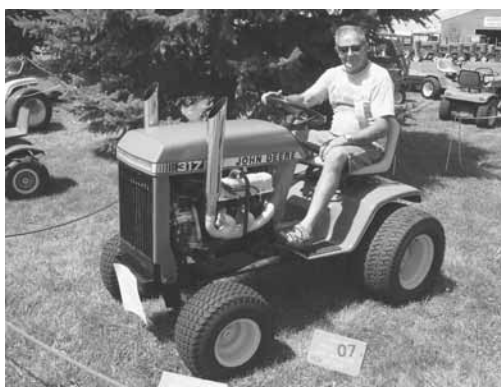
Pat Prom replaced the original engine in his Deere 317 garden tractor with a Buick 6-cyl. carbureted engine. "It has about 120 hp so it'll really go," he says.
