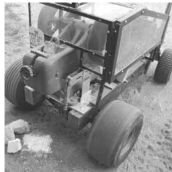
Larry Fulton's rock crusher was built for use in a minerals assay office in 1903. Fulton motorized the crusher and made it self-propelled as well.
