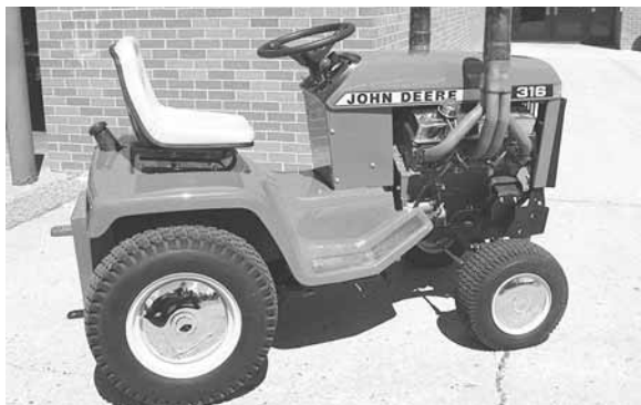
Students at the North Dakota State College of Science repowered this Deere 316 garden tractor with a 300 hp Chevy engine.
