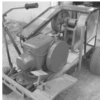
Larry Fulton's rock crusher was built for use in a minerals assay office in 1903. Fulton motorized the crusher and made it self-propelled as well.
