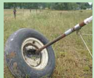
Electrified steel pipe with a swiveling pigtail holds the wire and has a plastic handle on top. Hochstetler uses the handle to roll unit to a new location with the electric wire still attached to pigtail.
