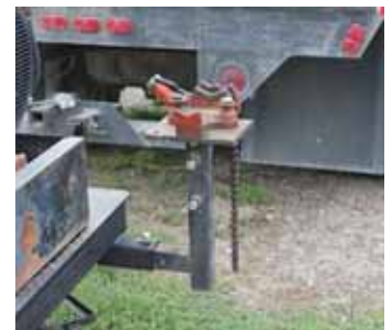
Dan Ambrose uses his home-built receiver hitch brackets on everything from welding trailers (above) to shop welding tables. “They allow me to use various tools interchangeably around my farm wherever I need them,” he says.
