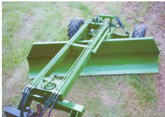
Pull-type grader hooks up to the 3-pt. hitch’s lower lift arms and is equipped with an oscillation joint that’s used to control the hydraulics and to roll the blade forward.
