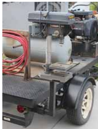
Dan Ambrose uses his home-built receiver hitch brackets on everything from welding trailers (above) to shop welding tables. “They allow me to use various tools interchangeably around my farm wherever I need them,” he says.
