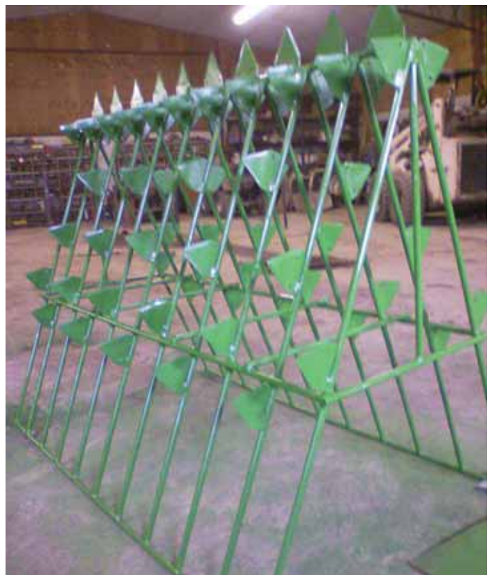
“Grain cage” consists of lengths of 1/2-in. dia. steel rod formed into a triangle, with sickle sections spaced about 5 in. apart welded onto the rods.
