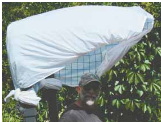
Mark Schecterson used an old bed sheet and some woven wire fencing to cover his Kubota loader tractor. The canopy measures 3 ft. square and mounts on tractor's rollbar.
