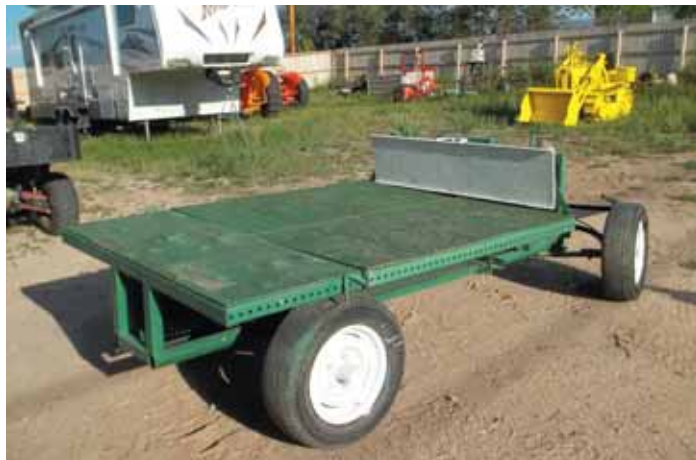
Larry Fulton’s flatbed trailer converts quickly to a 4-sided, belly dump wagon.
