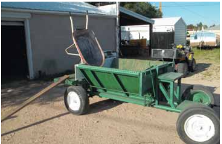
To dump, Fulton designed the wagon so 2 side panels on the bed tip in toward the center, forming the sides of the belly dump hopper.
