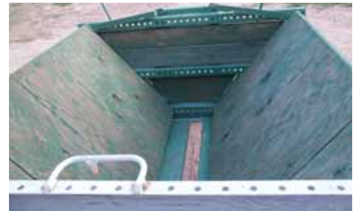
Fulton pulls on a lever to open two 9-in. sliding panels at bottom of hopper.
