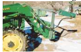
A length of pipe, with a pillow block bearing on one end and a hydraulic motor on the other, is used to hold the netting.
