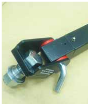
"Multi-axis" trailer coupler is designed to remain flexible on rough terrain without binding.
