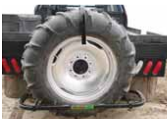
Rectangular metal frame attaches to pickup-mounted receiver hitch and uses a retaining arm to secure tire. Frame rotates down to the ground for loading.
