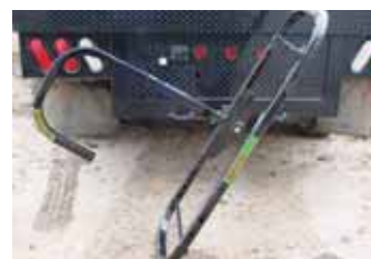
Rectangular metal frame attaches to pickup-mounted receiver hitch and uses a retaining arm to secure tire. Frame rotates down to the ground for loading.
