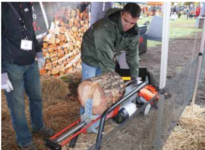
Electric splitter's C-channel design cradles log chunk and stabilizes the wedge as it travels through the wood.
