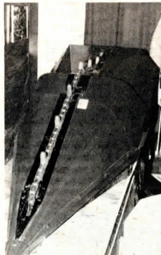
Conventional gathering chain picks up and carries down stalks to feeder auger.
