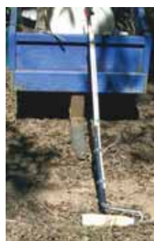
Robert Witt converted an electric paint roller into this wick wiper, allowing him to kill weeds right from his riding mower.
