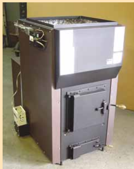
The Kuuma Vapor-Fire 100 hot air furnace recently tested out at 86 percent heat transfer efficiency, 98 percent combustion efficiency, and produced less than a gram per hour of particulates.
