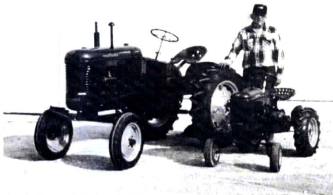
Massey Harris's hood and gas tank were made from an air conditioner freon tank.
