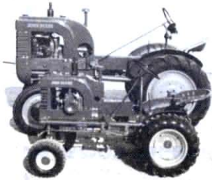
The Deere 4010 Hi-Boy is equipped with a narrow front axle. The half-scale antique tractor is geared down to permit very slow operation.
