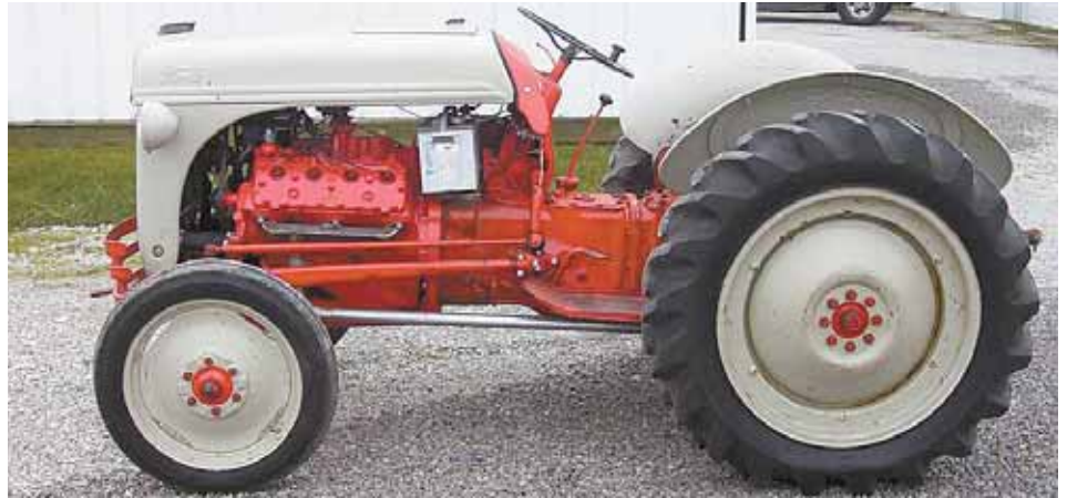
Kit costs $1095 and contains all the hardware needed to connect the V-8 engine and clutch assembly to the Ford 8N transmission and frame. Knasel says it takes about 8 to 10 hours to install.
