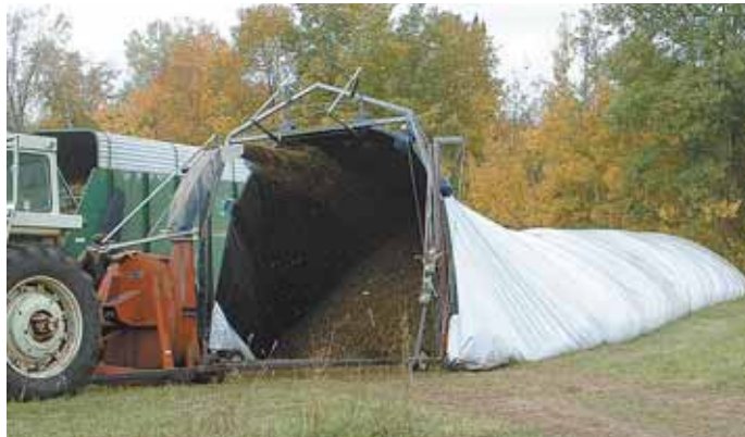
Wagons unload directly into blower. “New frame is higher and narrower to make a better packed bag,” says Walder.
