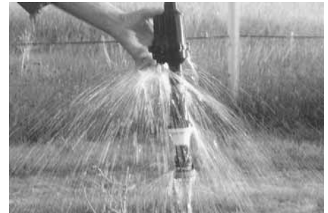
Filter fits between the hose and the regulator on center pivot drop nozzles (left). To flush out sediment you just push up a small release valve on side of filter.
