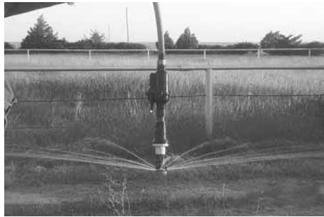
Filter fits between the hose and the regulator on center pivot drop nozzles (left). To flush out sediment you just push up a small release valve on side of filter.
