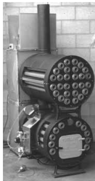
PapaBurn (with cutout sides to show heat exchanger tubes)
