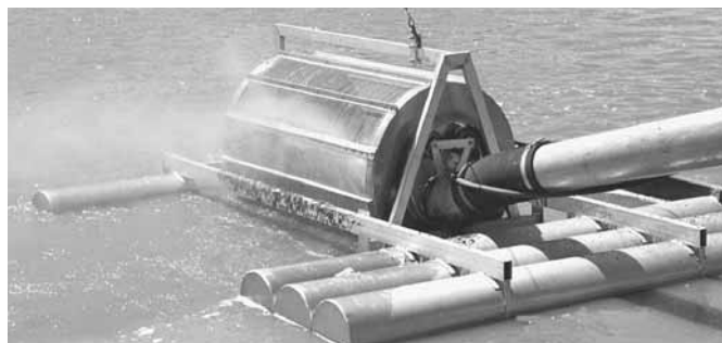
Water-driven, self-cleaning screen is designed to work in water as shallow as 4 in.
