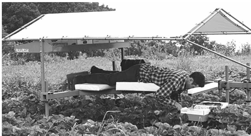
Battery-powered picking cart comes with a vinyl canopy that protects both the crop and the operator from sun or rain.
