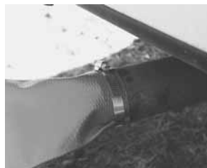
The “Critttergetter” kit (left) uses engine exhaust to kill gophers and other underground pests. Rigid plastic adapter (center) clamps onto vehicle’s exhaust pipe. An 8-in. long pvc tube (right) is used to get gas into tunnels.
