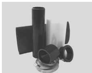
The “Critttergetter” kit (left) uses engine exhaust to kill gophers and other underground pests. Rigid plastic adapter (center) clamps onto vehicle’s exhaust pipe. An 8-in. long pvc tube (right) is used to get gas into tunnels.
