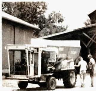
Schnittjer built his self-propelled feeder by mounting a stationary mixer box on a stripped-down IH 403 combine.
