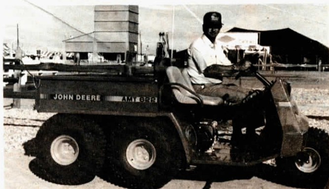
Deere's upgraded AMT has a steering wheel, two seats, a larger engine and more.
