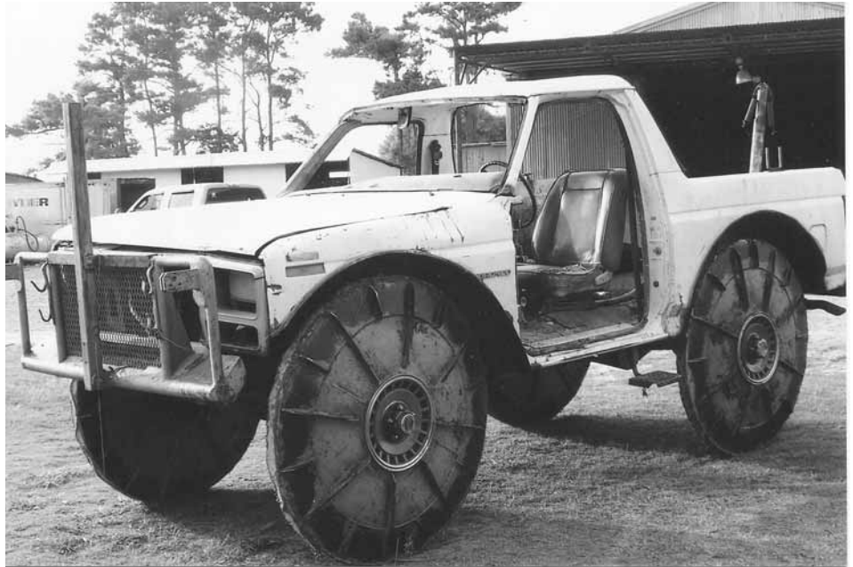
Big wheels increase rig's clearance from 10 to 24 in., which keeps truck from getting hung up in deep mud.
