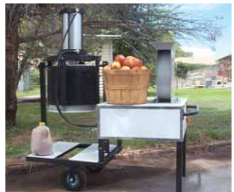
Frustrated with the small hand-operated cider presses on the market, Gerald Simons designed this model that can press out 20 to 25 gal. of cider per hour.
