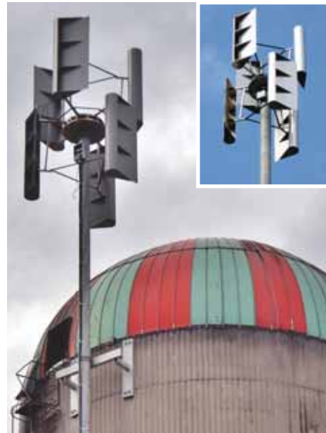
VBINE turbine can be mounted on its own pole or attached to an existing communications tower or even a silo.
