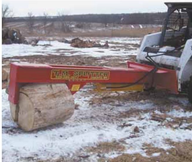
Log splitter is built from two pieces of channel iron mounted back to back, with an 8 by 24-in. “window” in between. The window design lets Trelstad see what he’s doing and is also stronger than a single I-beam.
