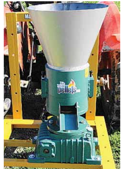
Pto-powered pelletizer has a heavier-duty gearbox that’ll stand up to increased pellet-making torque, says the company.
