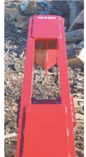
Log splitter is built from two pieces of channel iron mounted back to back, with an 8 by 24-in. “window” in between. The window design lets Trelstad see what he’s doing and is also stronger than a single I-beam.
