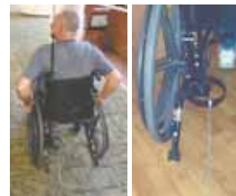
John Tierney says the "drag chain" he added to his hospital wheelchair stopped static shocks.
