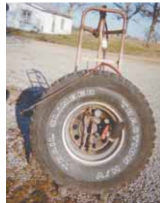
John Parker turned a truck wheel and tire into a sprayer to apply herbicide around his yard. Note pvc filler pipe on on tire rim.
