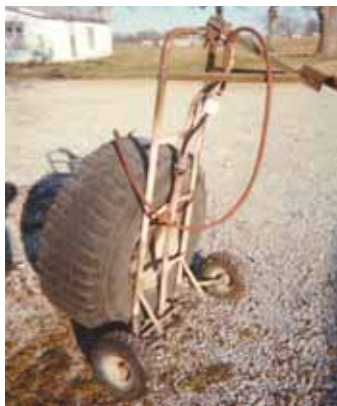
John Parker turned a truck wheel and tire into a sprayer to apply herbicide around his yard. Note pvc filler pipe on on tire rim.
