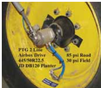
On-the-go tire inflation system makes it easy to adjust tire pressures on-the-go right in the field.
