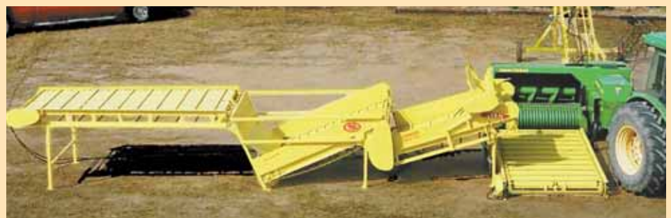
Simpson recently introduced a four-piece machine. While one bale is being unrolled for re-baling, you can load another bale onto the prep-table. When the first bale is done, you just flip a lever to advance another roll into the unroller chamber. (Unit shown is four-piece model.)
