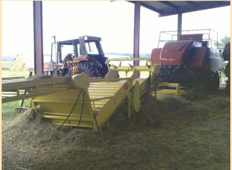
As roll is turned, hay is fed into large square baler similar to a small baler.
