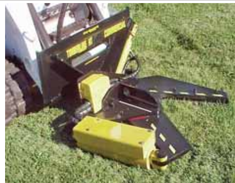
Model HTC-14 can cut a 14-in. tree at ground level in 5.5 seconds. All major pivot points are machined and greaseable for long life.
