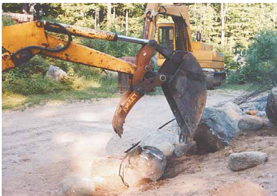
Hoe Clamp moves as bucket moves. Lund says it's easier to use than a "hydraulic thumb".
