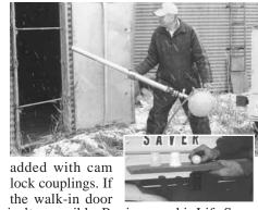
isn't accessible, Perrion uses his Life Saver from the top of the bin. He slips in an ice cube and holds it in place with a paper straw slipped through a 1/4-in. hole drilled through the pipe.
