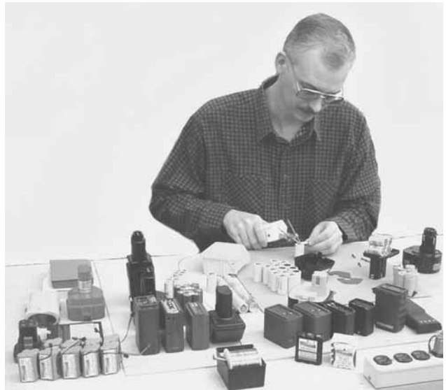
Primecell has developed a way to open batteries to replace the cells, then reseal them without damage.
