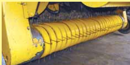
Pickup fitted with new Tobin poly bands.
