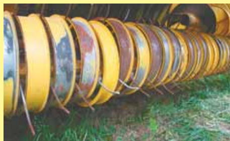
Baler pickup with bent, rusted steel bands.
