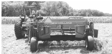
**The amount of moisture in the crop does not affect operation of the rubber-coated rollers, says the company.**
