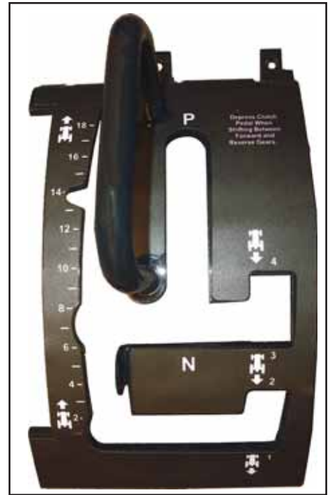
Shift kit includes a lock lever that blocks off the lower 6 gears to shorten up your shift movements.
