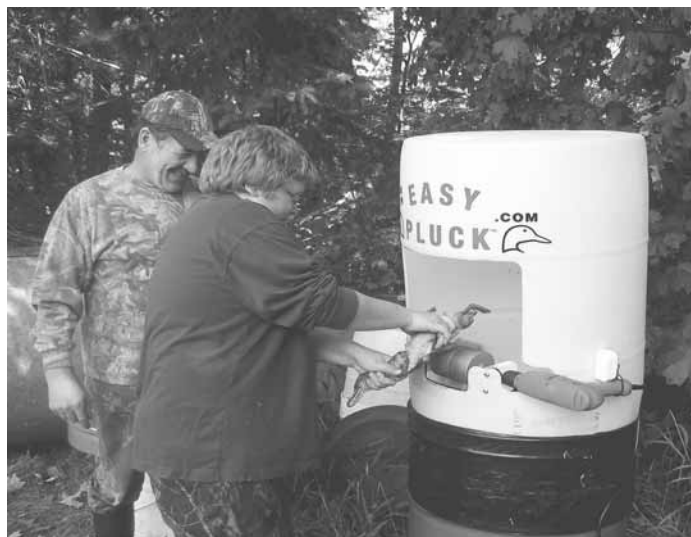
Easy Pluck mounts inside a 55-gal. plastic barrel, which catches all the feathers. Unit is driven by a 3/8-in. power drill.
