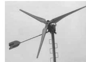
Win-Pressor turbines are designed to produce compressed air instead of electricity. Photo at upper left shows unit in gear. Photo at lower left shows unit furlled and out of gear.
