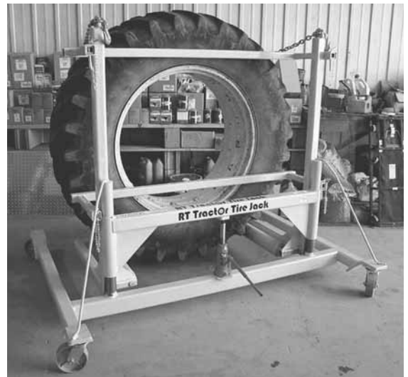
Tire jack uses a pair of adjustable arms to quickly and easily remove large tractor tires.
