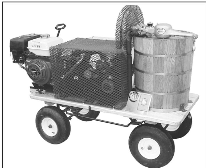
**Machine's 5-gal. can is lined with copper coils, which cools the ice cream and eliminates the need for salt or ice.**
