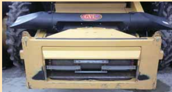
EZ-View Dust Diverter can be installed in 30 min. or less and the ends flip up for easy cleaning.
