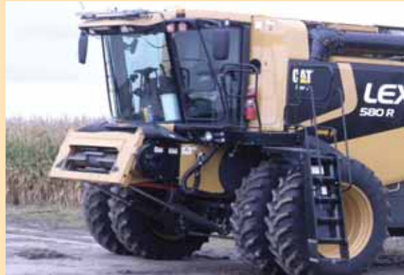
GVL's "no hydraulics" Dust Diverter was engineered to fit the new Lexion Header Pitch feederhouse.
