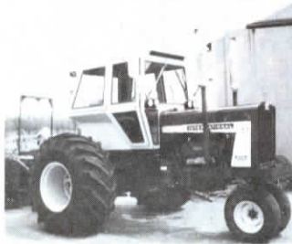
Carroll repowered this IH 806 tractor with a 504 Cummins engine.
