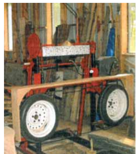
In 2010 Reeks designed his latest new sawmill, the Thriftwood. It's powered by a single phase 220-V motor. No fumes so it can be used inside.
