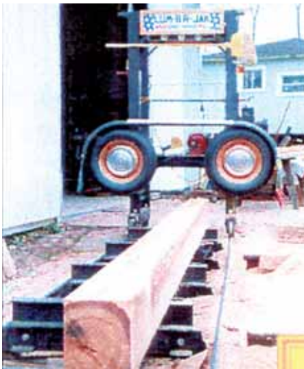
Reeks first sawmill, the Lum-BR-Jak, was built in 1994 from miscellaneous parts for less than $100.
