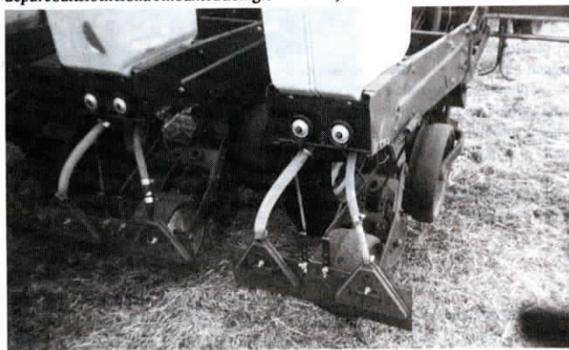
Blonigan mounts pairs of row banders behind each row at back of planter.
