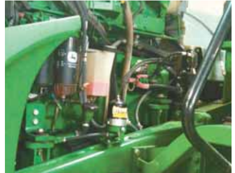
Photo above shows a Dieselcraft unit installed on a Deere 9430 tractor. Photo at left shows a unit on a Cat D6H.
