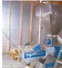
Separated dairy manure solids are put through a screw-type press. "Finished" compost is crated, ready for shipping to buyers.
