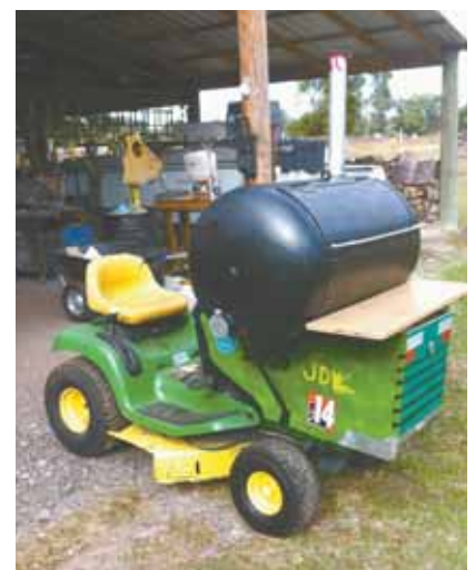
A modified 60-gal. air compressor tank mounts on top of Deere LT 133 tractor.
