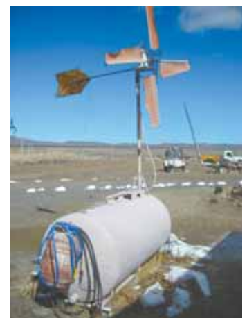
Jeff Hoard uses a homemade windmill to compress air that's stored in a 400-gal. propane tank.
